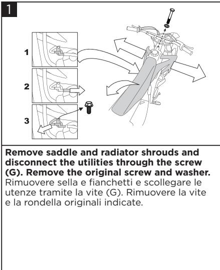
**Remove saddle and radiator shrouds and disconnect the utilities through the screw (G). Remove the original screw and washer.**
