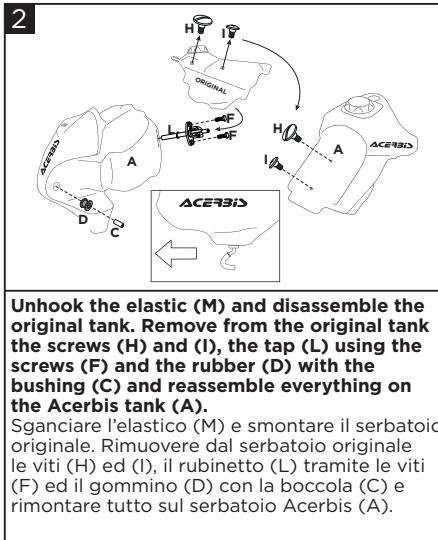
**Unhook the elastic (M) and disassemble the original tank. Remove from the original tank the screws (H) and (I), the tap (L) using the screws (F) and the rubber (D) with the bushing (C) and reassemble everything on the Acerbis tank (A).**
