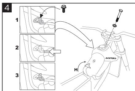
**Hook the elastic (M), connect the utilities using the screw (F) and reassemble the original plastics. Mount the screw (B) with the washer (E).**
